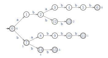
Insertion of u = y[i ... n - 1] in the structure accepting longer suffixes
